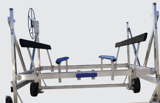
Spring loaded (14' vertical) full length guide-ons of carpeted wood is less likely to damage decals, a must for inboard boats.
