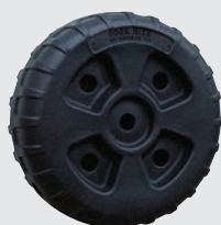
Molded Polyethylene Wheel with an 800lb capacity cannot go flat. The large diameter, wide wheel rolls better and will sink less, making installation and removal easier.
